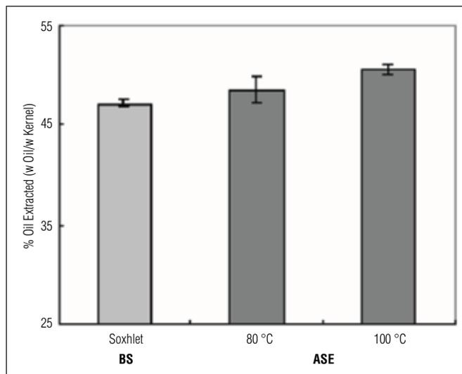
Figure 1. Percentage of oil extracted using the British standard and ASE method.
